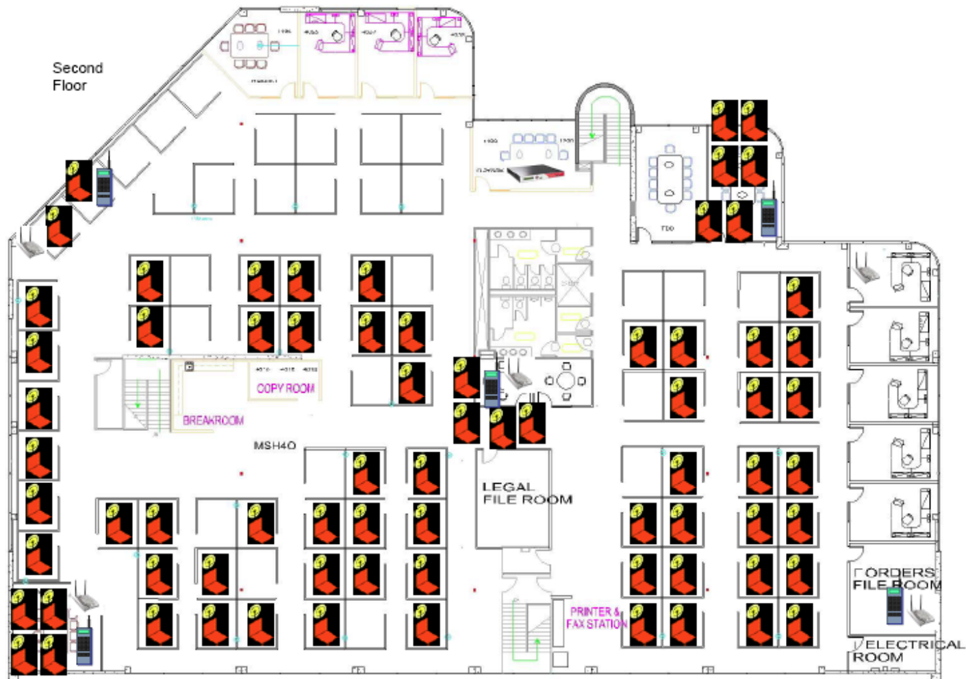
Figure 1 – Schematic diagram of the equipment layout used in this testing. All locations of equipment are approximate. Each orange notebook icon represents a single wireless notebook. Each telephone icon represents ten VoFi handsets. Each AP icon represents three APs, one on each of channels 1, 6, and 11. The Meru MC3000 controller was located in the conference room in the center top of this drawing, connected to the APs via switches located on the first floor. Source: Farpoint Group.
